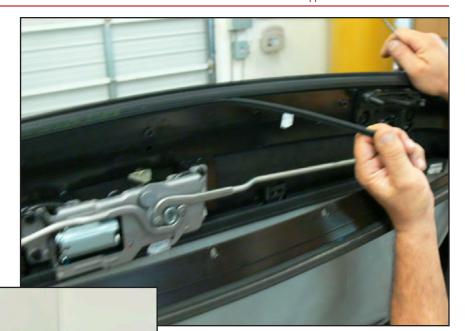
**5** Use a flat-head screwdriver to pry out and remove header extrusion from header bow.
