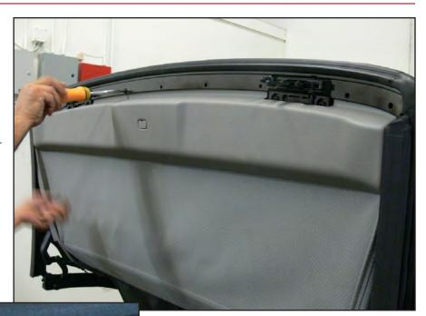
**32** Rivet to secure side support straps to frame.
