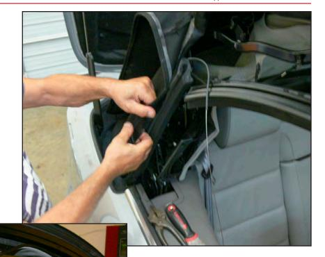
**11** Remove headliner extrusion from bottom rail.
