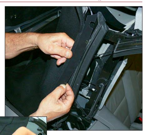
**26** Transfer original clips to Top rear plastic retainer, insert retainer into bottom rail and force to lock.
