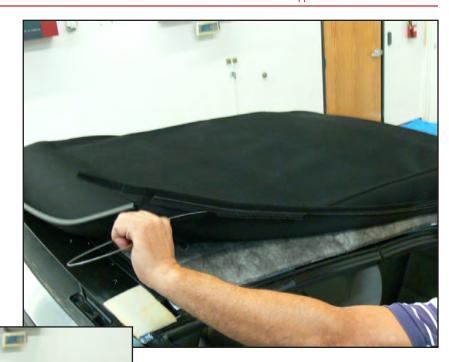
**23** Attach tension cable ends to Top frame.
