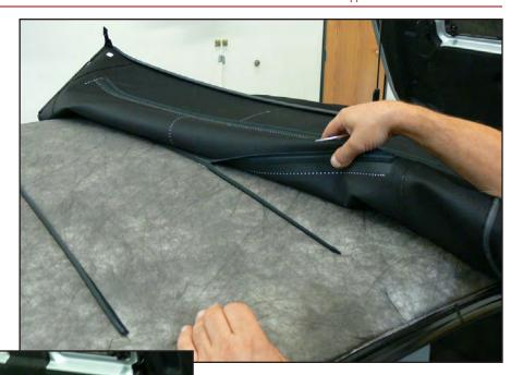
**8** Pull out tension cables from Top sleeves (left & right).
