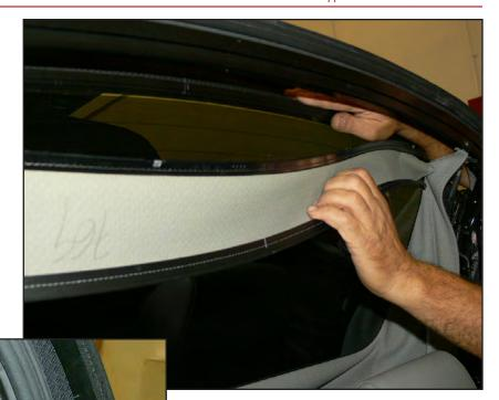
14 Disconnect left & right defroster leads. Cut zip tie and open cover to release defrost wire, and then unplug connector.
