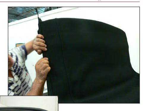
**29** Position weather seal retainer to header.
